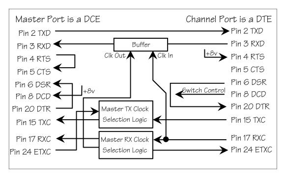
Master DCE / Sub-Channel DTE Interface Flow Diagram
